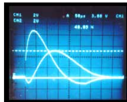
Center Conductor "Surge" Delay can damage equipment
