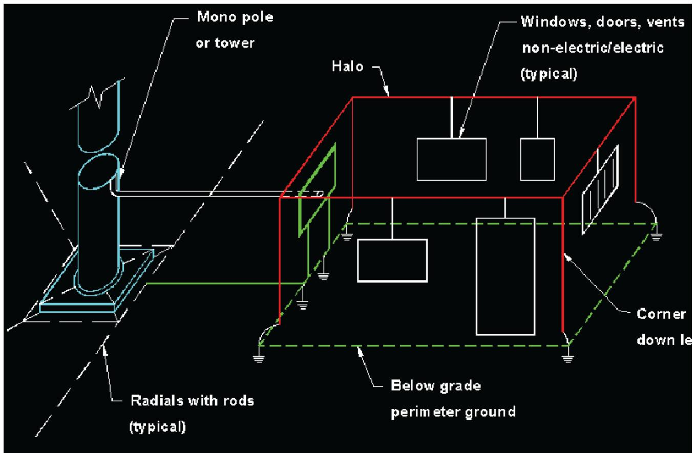
(1) The halo should not be interconnected with or used as a ground connection for any active electronic equipment. Do not attach the halo to the single point ground, equipment racks or the entrance panel / bulkhead / hatchplate / coax line ground bar.
