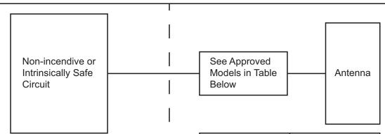
Note 1: Non-incendive field wiring to be installed with NEC Article 504.
