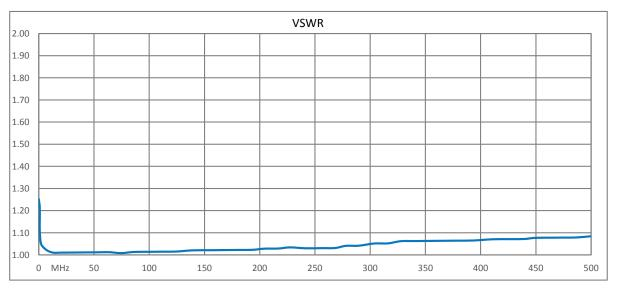
Click the following link (or enter part number in "SEARCH" on website) to obtain additional part information including price, inventory and certifications: UHF F/M Coaxial RF Surge Protector, 50MHz - 700MHz, DC Block, 375W, 600uJ, 50kA, Blocking Cap, Bracket Up, Hole Mount IS-50UX-C1-ME
