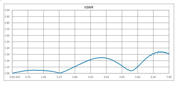
Click the following link (or enter part number in "SEARCH" on website) to obtain additional part information including price, inventory and certifications: TNC F/M Bulkhead Coaxial RF Surge Protector, DC - 7GHz, DC Pass, 90W, IP67, 4mJ, 20kA, Gas Discharge Tube GT-TFM-AL
